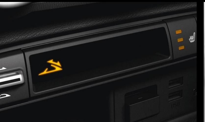
GUMB ZA OTVARANJE/ZATVARANJE KROVA (IZVEDBA RF)
